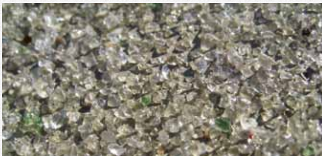
The tumbled glass grains as pre-applied surface material produces the high skid resistance.
